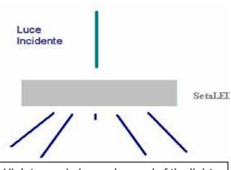
High transmission and spread of the light eradiated from the source. Effectiveness of the banners and no visible hot spots.
