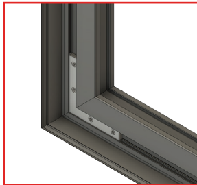
CORNERS Connect with TEXCORNs (use on each side)
