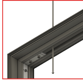
SUSPENSION Drill hole and use suspension cable with ball
